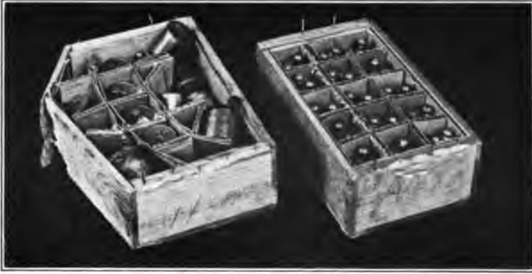
GRENADE BOXES WITH LOOSE- (ON LEFT) AND TIGHT-FITTING CELLS AFTER TEST
